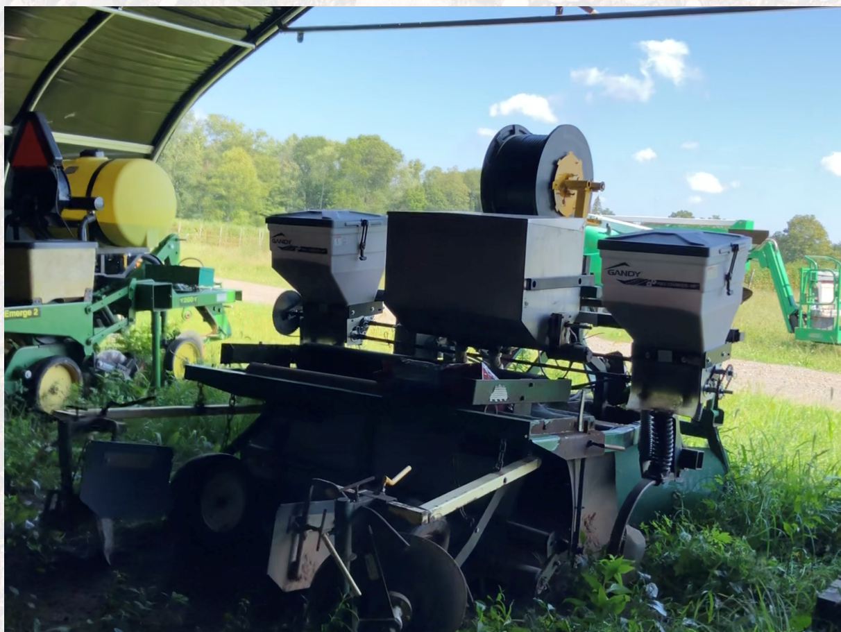
Addition of seed hoppers to the 2600 Rain-Flo Plastic Mulch Layer to seed cover crops on both sides of the plastic bed where soil would remain bare otherwise.
