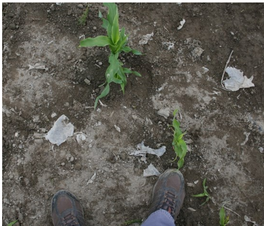
Fig. 1. Oxo- and photo-degradable plastic includes additives that cause the material to turn brittle and break into fragments when exposed to UV light, heat, and/or oxygen.
