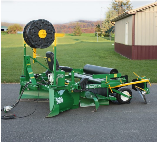
Figure 2. Mulch and drip tape can be laid simultaneously; note the round drum of drip tape on the left above, and the roll of mulch on the right.
