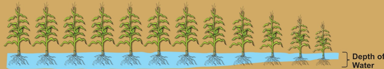
POOR UNIFORMITY- Dripline Length-of-Run Too Long
