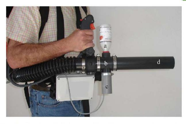
Fig. 1 — Mechanical blower: a) bottle containing beneficial organisms; b) extraction system; c) electromagnet; d) air diffuser.
