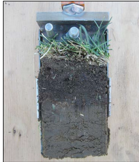
Figure 10. Compost topdressing is extremely difficult to incorporate into the existing soil. Topdressing should coincide with aggressive hollow-tine cultivation to mix the compost as much as possible with the existing soil. However, a topdressing layer is still likely to form, as seen above.
