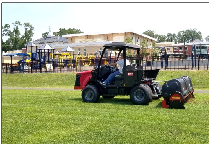
Figure 4. Use only Power Take-Off (PTO) driven, vertically-operating, core cultivation units. These units can provide consistent penetration depth to 3-4". Avoid drum-type core cultivators whenever possible due to their shallow, inconsistent penetration depth. Photo by Alyssa Siegel-Miles.
