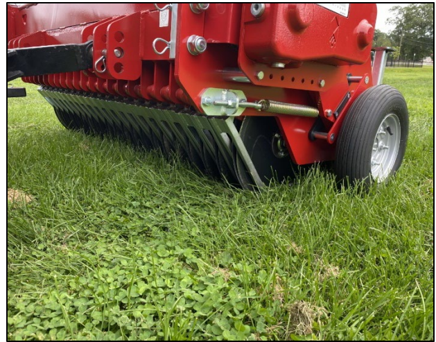
Figure 9. In the absence of imminent cleated traffic, seed should be applied using a spike seeder that will maximize seed to soil contact while minimizing damage to the existing turfgrass stand.
