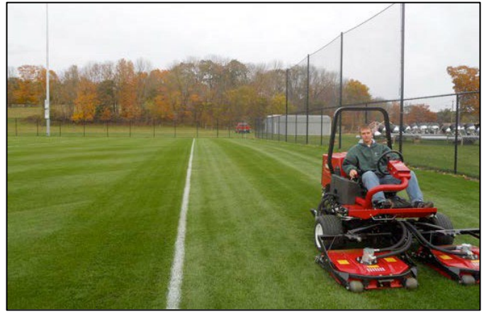
Figure 2. Consider using rotary mowers with contour decks. These mowers are easier to maintain than reel mowers, provide a high quality cut, disperse clippings very well and stripe nicely.
