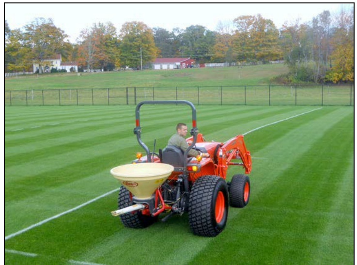
Figure 3. Consider using high capacity broadcast spreaders to cover large areas quickly.
