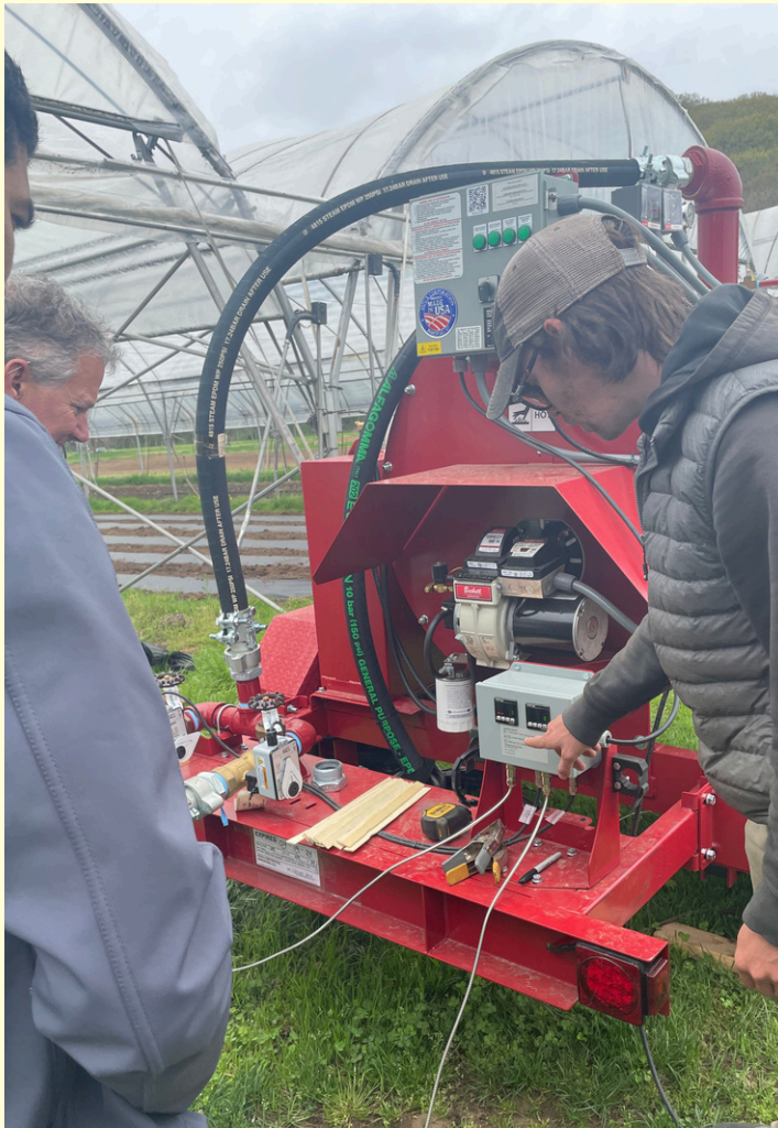
Photo 2: A closer look at the soil steaming technology of this Sioux Steam-Flo model.
