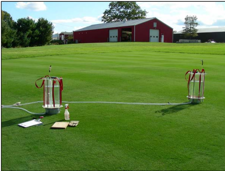
Figure 9. Infiltration rates were quantified in 2009 using a rain simulator developed by Ogden et al. 1997.
