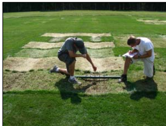
Fig. 2. Displacement readings being taken using a custom designed apparatus
