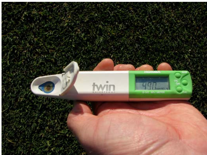
Fig. 9. Cardy nitrate sap meter. Left-side of meter shows collection well, where sap is placed on membrane for direct nitrate analysis. Digital reading is shown in the display on the right.
