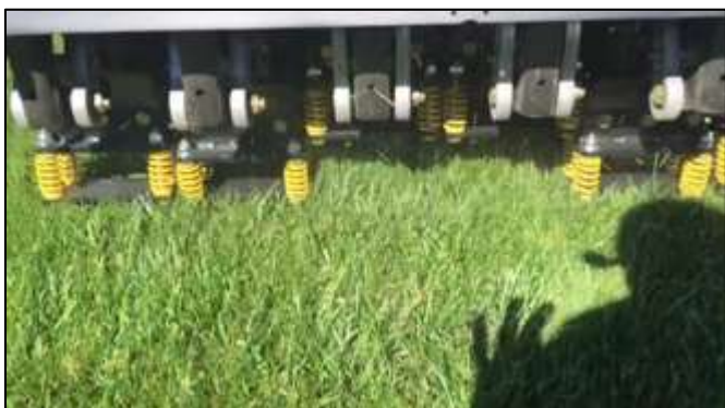
Figure 2. Modified greens aerator used to simulate traffic on athletic playing fields.
