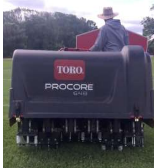
Figure 1. Modified greens aerator used to simulate traffic on athletic playing fields
