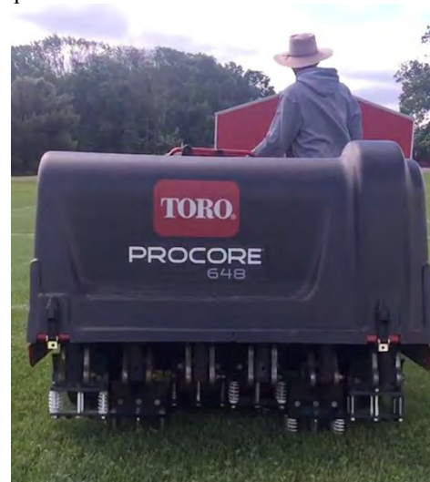
Figure 1. The Cady Traffic Simulator was used on the athletic field research area to simulate traffic.
