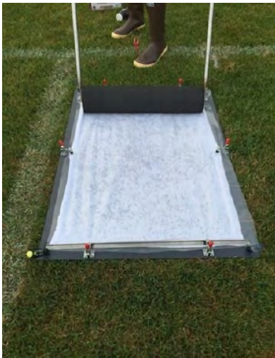
Figure 2. Cloth sample after being rolled. Dew moisture visible on cloth.
