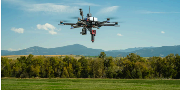
Figure 10. Drone equipped with hyper-spectral sensors (Vision Aerial, 2023)
